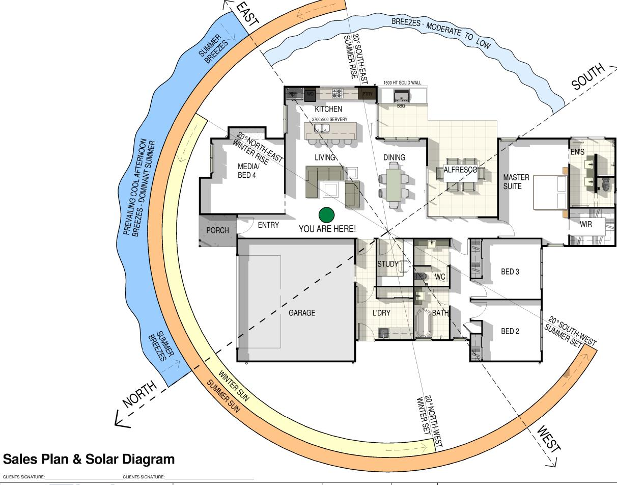
CLIENTS SIGNATURE: DESIGN: JOB ADDRESS: JOB NO: STAGED PLAN: PROPERTY DETAILS WORKING DRAWINGS **INNOVATION HOUSE** -USE FIGURED DIMENSIONS AT ALL TIMES. REFER ANY ENQUIRES TO BUILDING CONTRACTOR. ALL DIMENSIONS TO BE VERIFIED ON SITE PRIOR TO CONSTRUCTION. ALL WORK SCALE: ISSUE: 1:100 **STANDARD** Ε DRAWN: CHECKED: DWG NO: TO COMPLY WITH LOCAL AUTHORITY REGULATIONS AND BCA. **FINLAY HOMES** 03.07.13 DH BJC 202
